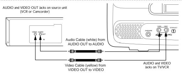
Make the connections shown above, using audio and video cables. Make sure the source unit (VCR or camcorder) is connected to a power source.
